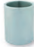
THREADED GLAND NUT ADAPTOR to weld to strut tube FH8021 ID 49.6mm / length 75mm Use KONI gland nut 7325-01-0071
